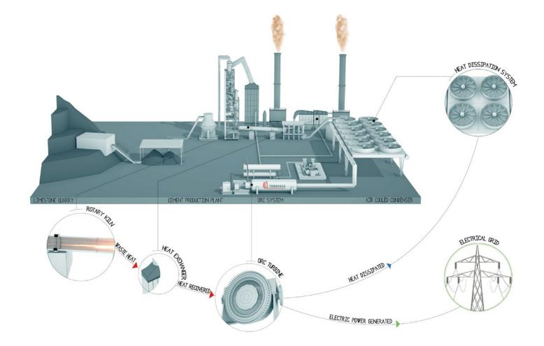
Example of a cement production plant integrated with a Turboden ORC system.
