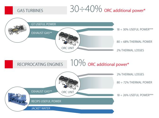
\* ORC power output compared to GT or RECIPS shaft capacity (e.g. 10 MW GT  $\rightarrow$  3÷4 MWe ORC). \*\* Min. flow to ORC: 10-15 kg/s.
