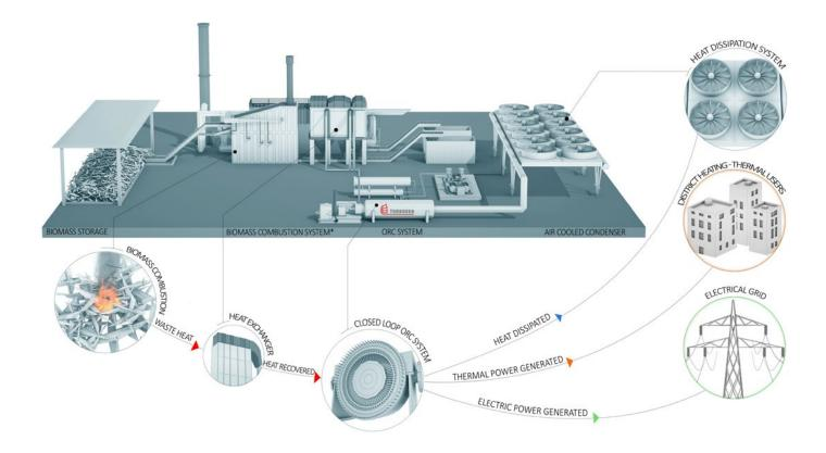
Example of a biomass plant integrated with a Turboden ORC system.
