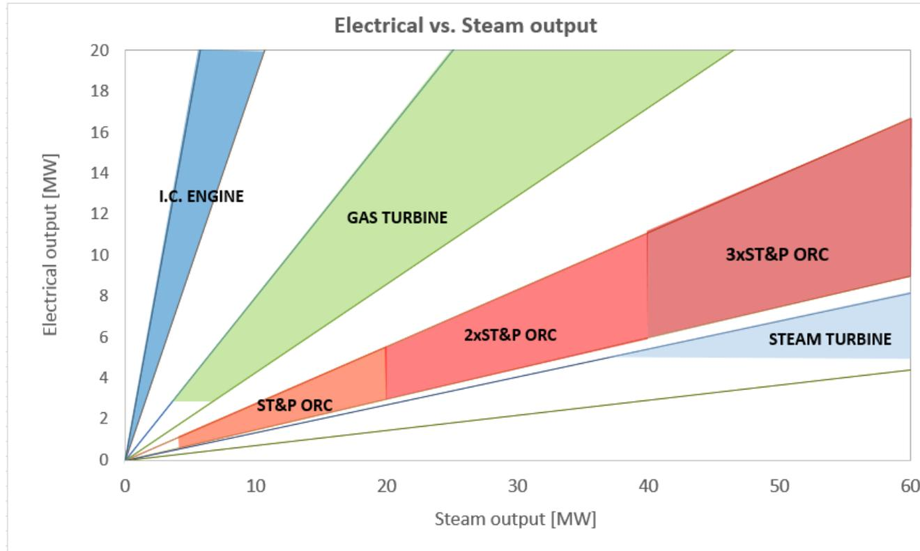
Each CHP technology (e.g. internal combustion engines, gas turbines, high-temperature CHP, etc.) has its own specific production characteristics in terms of steam and electricity productions.
