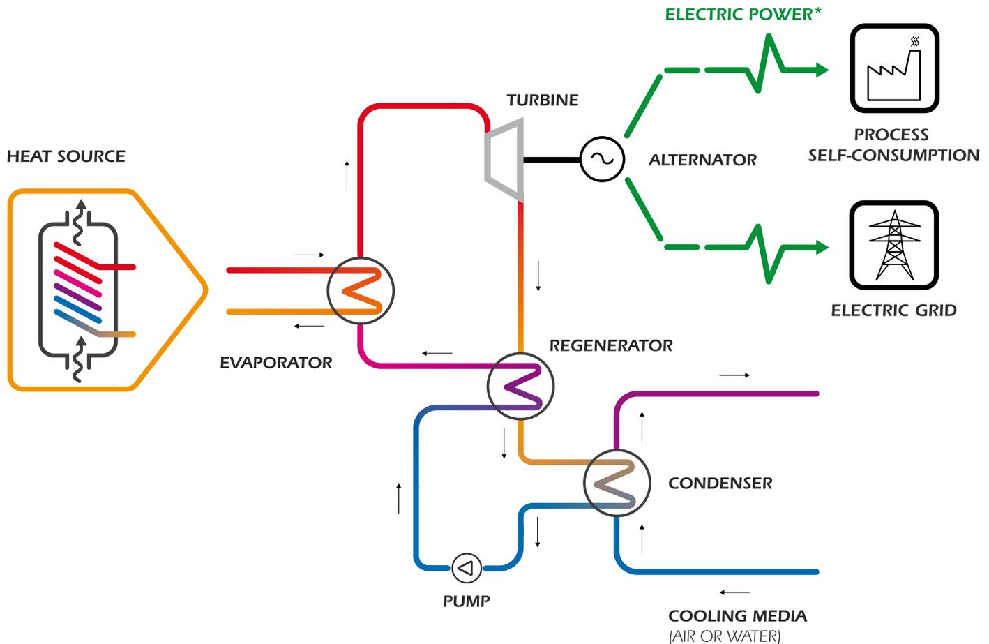
\* ORC units can produce electric and/or mechanical power
