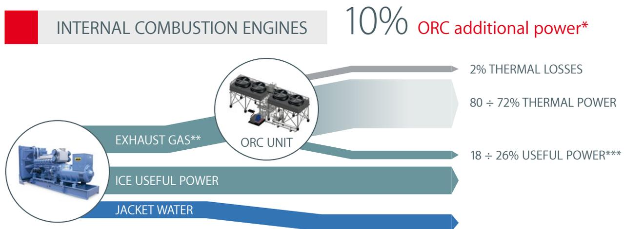
\* ORC power output compared to GT or ICE shaft capacity (e.g. 10 MW GT → 3÷4 MWe ORC).
