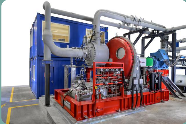
Integrally geared compressor double stage overhung
