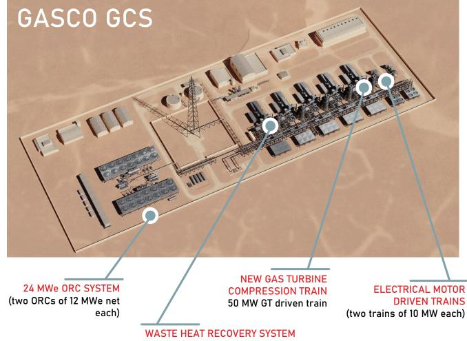
WASTE HEAT RECOVERY SYSTEM one WHR exchanger for each GT (4 existing GTs + 1 new GT)
