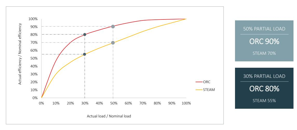
NOTE: steam turbine suffers partial load operation due to high risk of blade erosion.
