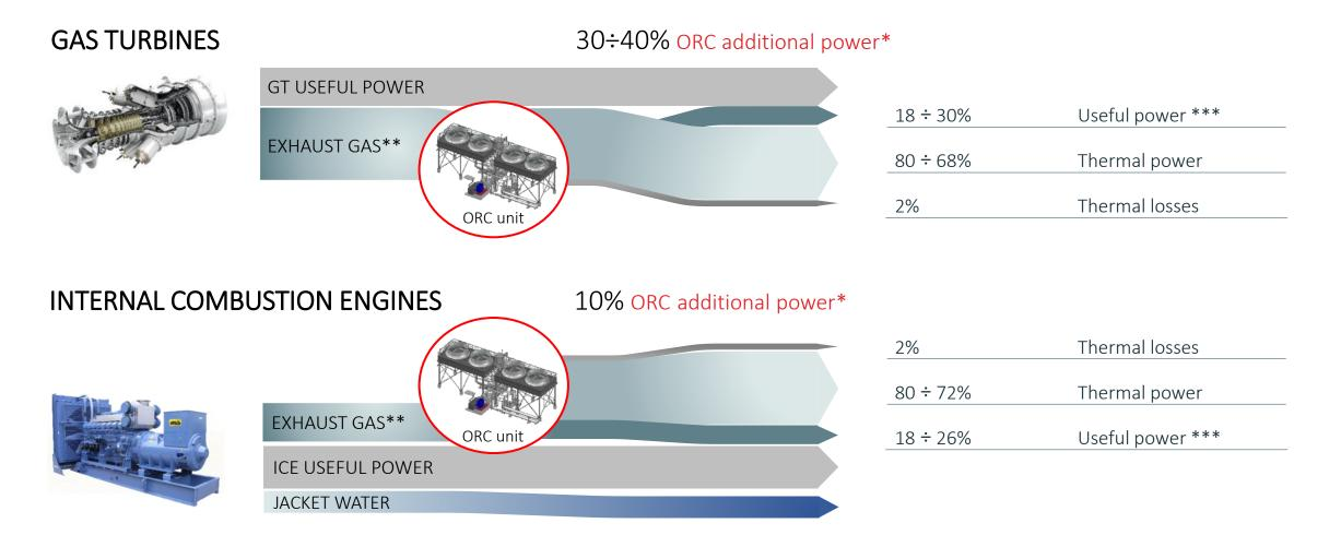
\* ORC power output compared to GT or ICE shaft capacity (e.g. 10 MW GT  $\rightarrow$  3÷4 MWe ORC; 10 MW ICE  $\rightarrow$  approx. 1 MWe ORC).
