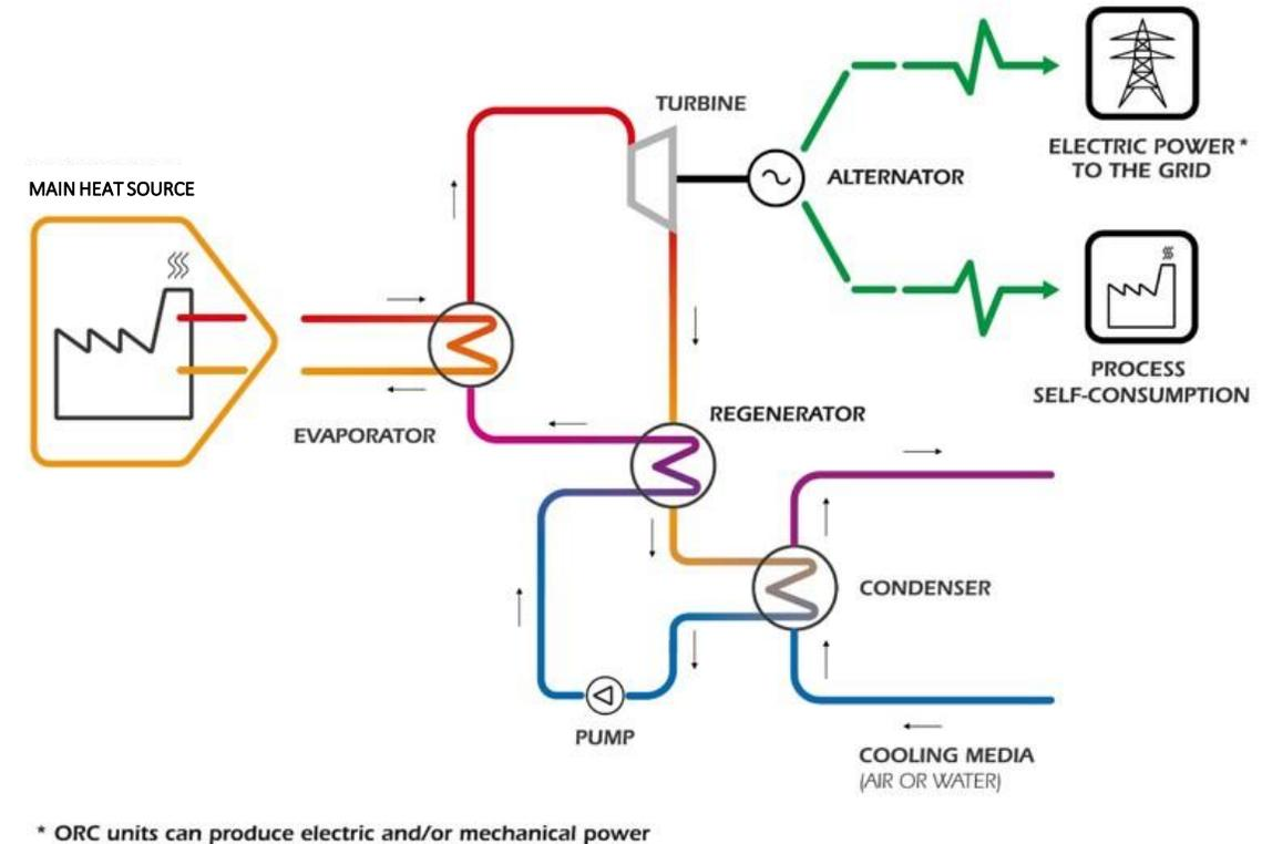
The waste heat from production process is transferred to the ORC working fluid by means of an intermediate circuit or directly via the exhaust gases in direct exchange systems. The media used in the intermediate circuits are thermal oil, saturated steam or superheated water.
