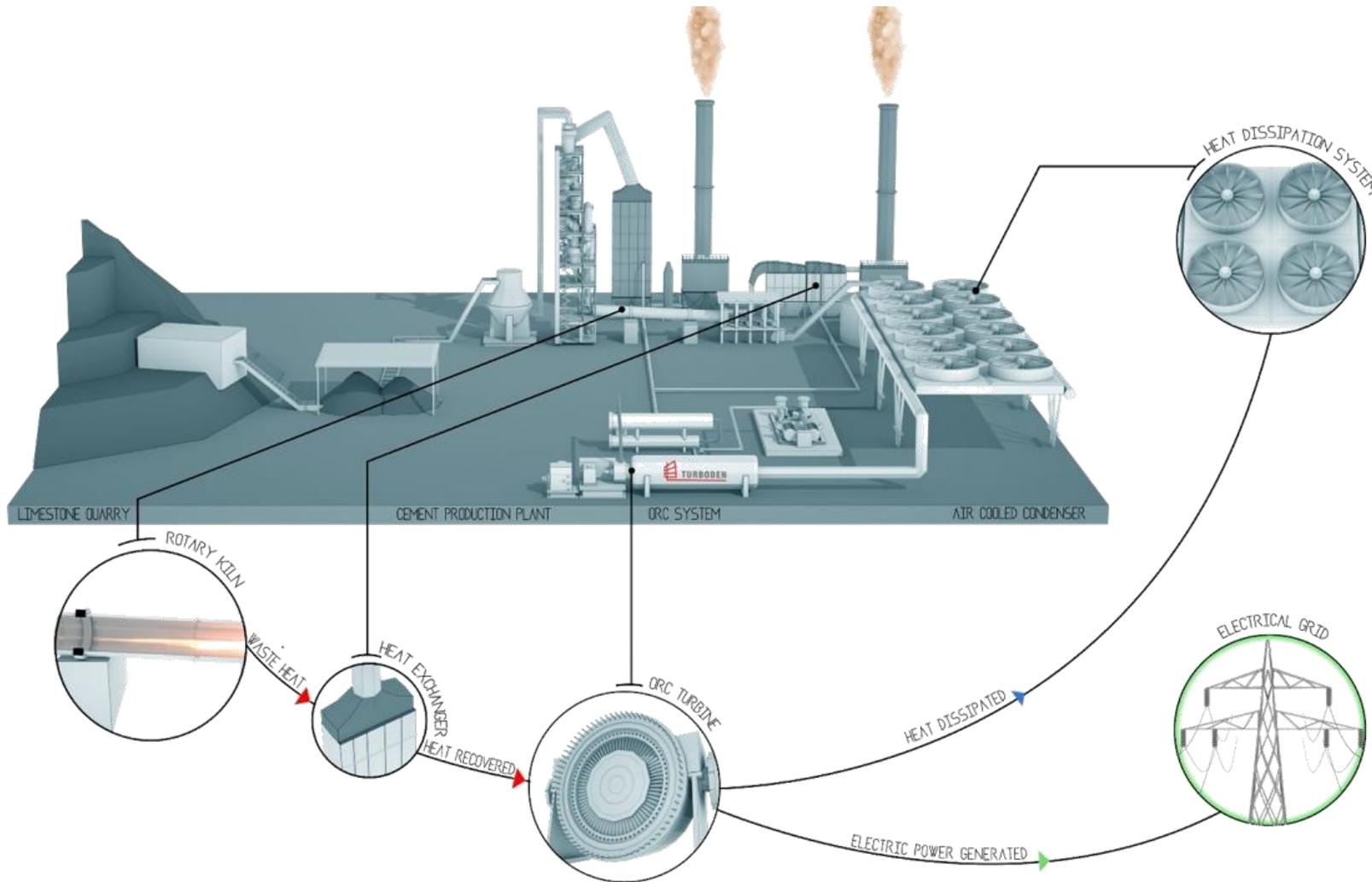
In cement production process, Turboden ORC systems can produce electric power by recovering waste heat from two hot gas streams:
