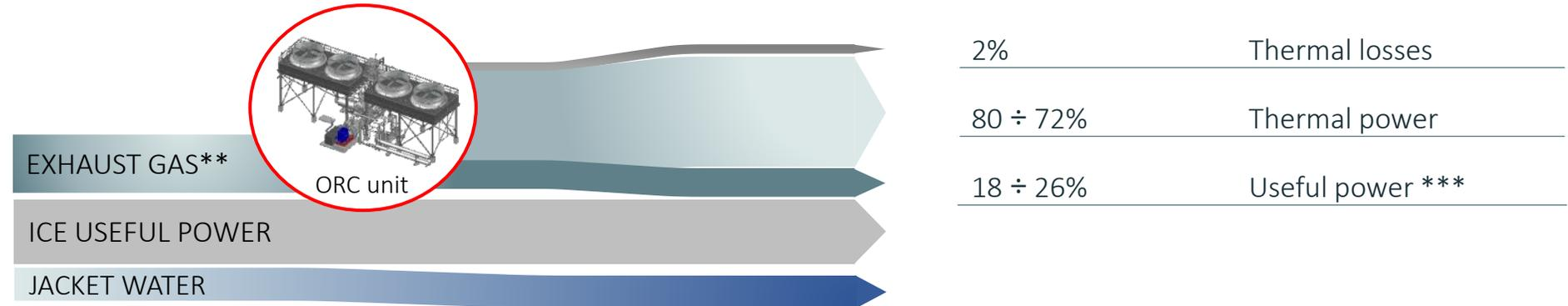
\* ORC power output compared to GT or ICE shaft capacity (e.g. 10 MW GT → 3÷4 MWe ORC; 10 MW ICE → approx. 1 MWe ORC).
