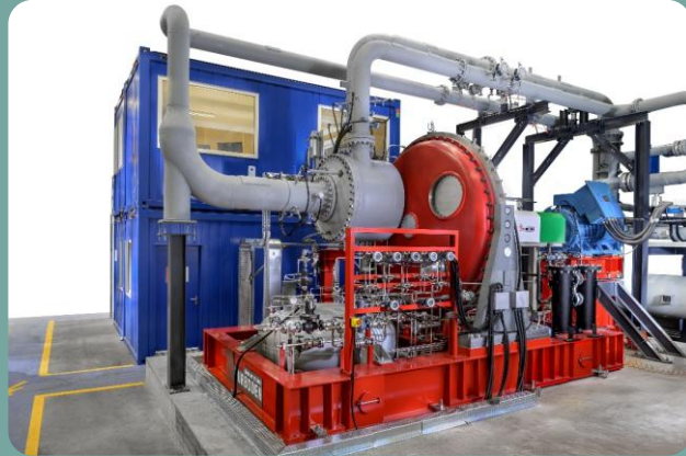
Integrally geared compressor double stage overhung
