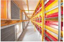
The Güres Group has developed a newgeneration manure dryer to run with a lowtemperature heat source, such as 70-degree water Contributed photos
