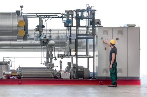
are already in operation in Saint-Gobain Italy. In this case the turbine is connected to a double shaft generator that is connected to the compressor. About half of mechanical power (500 kW) is transformed into electricity, while the rest is used to produced 80 Nm<sup>3</sup>/min at 7 bar(g) (*Fig 2*).
